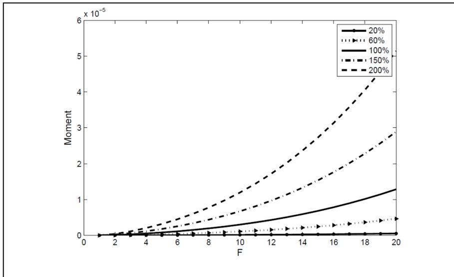
Fig.(4). Change in the variance (second-order central moment)  $\mu_2$  of the top-event probability Q due to identical variations in error factors of all  $q$ 's.
