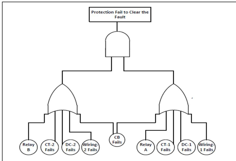
Fig. (2). Fault-tree diagram for a redundant system.
