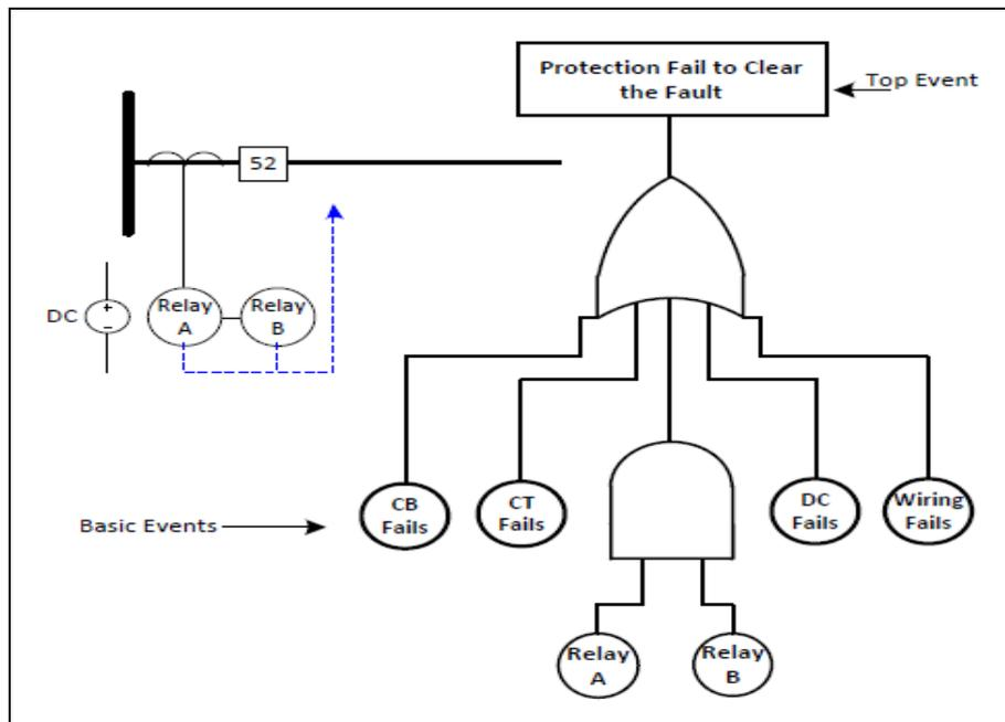
Fig. (1). Relay one-line diagram with corresponding fault-tree diagram.
