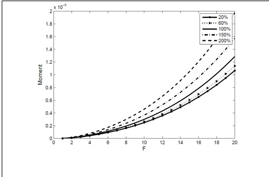
Fig. (3). Change in the variance (second-order central moment)  $\mu_2$  of the top-event probability Q due to variation in  $q_1$  error factor alone.
