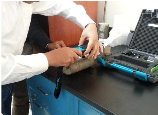
**Fig. (2).** Electrical resistivity test.
