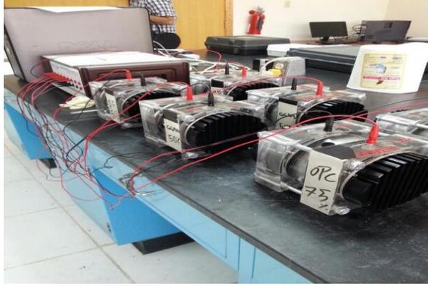
Fig. (3). Rapid chloride permeability test cells
