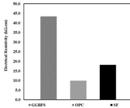
Fig. (6). Electrical resistivity for OPC, SF and GGBFS concrete
