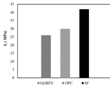
Fig. (5). Compressive strength for OPC, SF, and GGBFS concrete
