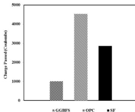
Fig. (7). Rapid chloride permeability of OPC, SF and GGBFS concrete
