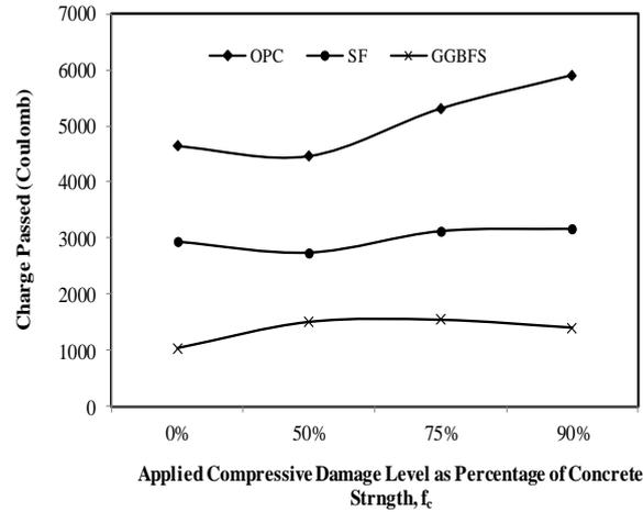
Fig. (9). Effect of compressive damage on RCPT of concrete
