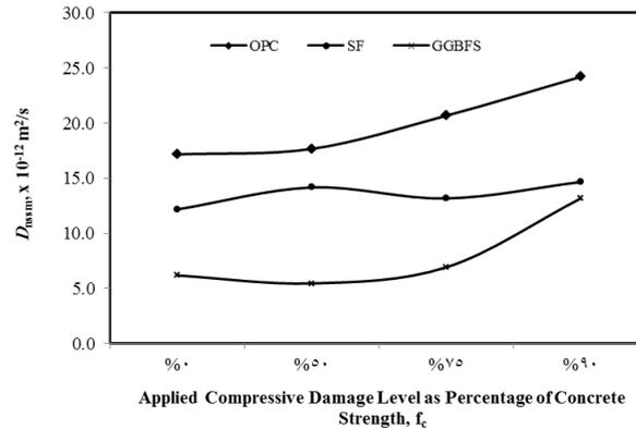
Fig. (10). Effect of compressive damage on chloride migration coefficient
