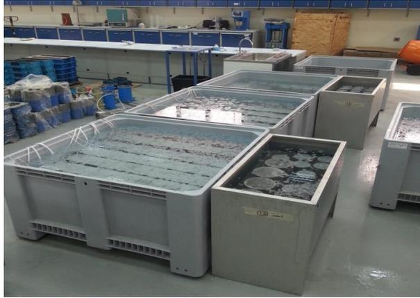
**Fig. (1).** Concrete samples in the curing tanks
