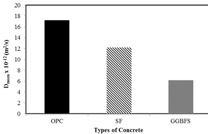
Fig. (8). Chloride migration coefficient in OPC, SF, and GGBFS concrete
