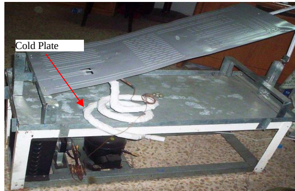
Fig.(2). Photo of the test rig components.
