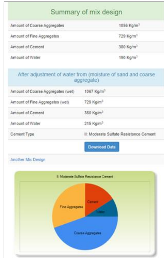
Fig. (21). Output results of the software for example (3) (Concrete mixture design)
