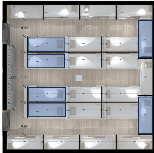
Fig (8). Install six beds that are two metres in length.
